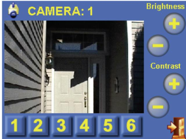
The top line displays the camera number that you are currently viewing (i.e. CAMERA: 1).
