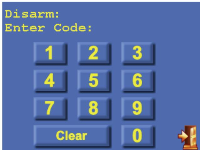
Enter your four-digit code. If you make a mistake, press the [Clear] button and start over or press the [exit] button to return to the previous page. After the last digit of a valid code is entered, the system will perform the desired task.
