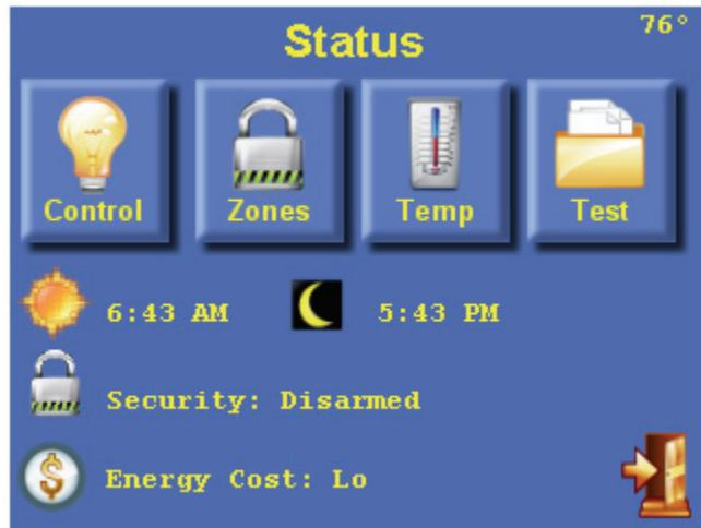
The main “Status” page displays the time of Sunrise and Sunset for the current day, current security mode, energy cost, and outdoor temperature (if applicable). According to your system configuration, not all icons may be visible (as shown above).
