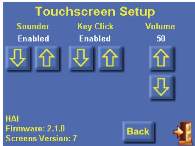
When complete, press [Back] to return to the previous setup page or the [exit] button in the lower-right corner to save the settings and exit (back to the Home page).
