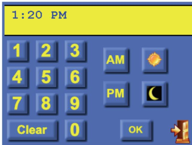
Enter the time (use either AM/PM or 24HR time format). Press the [sun] button for the “time of Sunrise” or the [moon] button for the “time of Sunset”. Once complete, press the [OK] button to save time. If you make a mistake, press the [Clear] button and start over.
