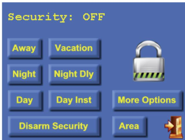
The top line on the “Security” page displays the current security mode.
