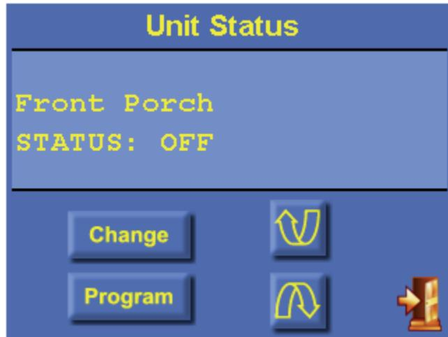
Press [page down] to display the next item and press [page up] to display the previous item. Press the [Change] button to change the status of the selected device.
